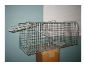
Figure 35, Collapsible cage trap with treadle
