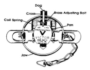
Figure 1. Anatomy of a double coil leg-hold trap
